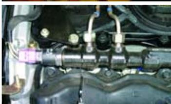
The tuning module was connected to the common-rail system via the wiring loom and attached to the bulkhead
